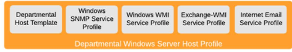
At the next level of abstraction, host profiles are the combination of a host template and one or more service profiles. For example, you can have a generic "Windows Server" host profile that combines a generic host template with service profiles for system-level SNMP and WMI lookups,
